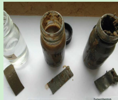
Test result: No corrosion due to sugar beet silage
