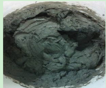
Maleki-SWP 270 after mixing with water before maturing.
