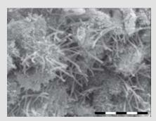
Typical cement matrix (23 μm)
